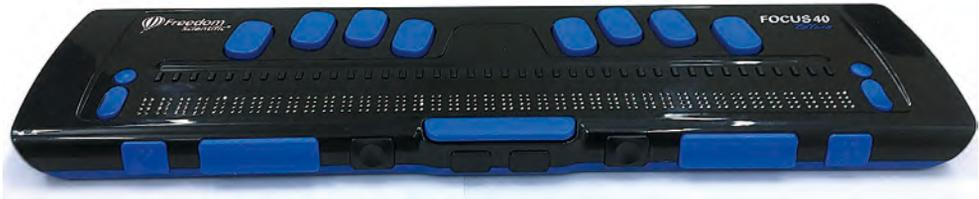
Figure 14.6 A braille keyboard with a small reading display
